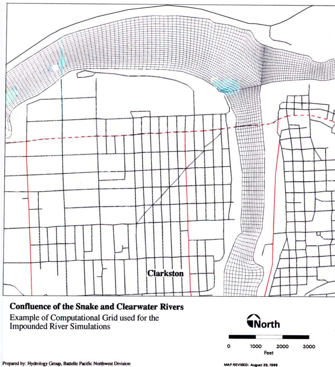
Figure 8-1. Example of the Computational Grid Used in the Full-pool, Impounded Conditions Simulations
